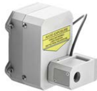
Attenuator AT1 and pulse energy monitor EM1
