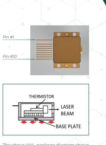
The above HHL-package diagram shows the built-in thermistor that monitors the laser chip temperature. The diagram also shows the base plate that dissipates the heat generated by the TEC and the laser chip.
