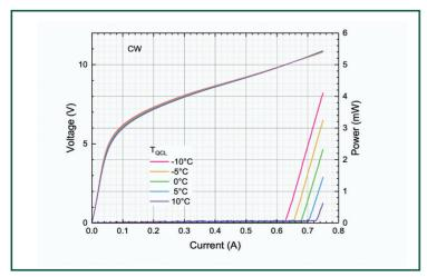
Single Mode Distributed Feedback Quantum Cascade laser at ~628 cm-1
