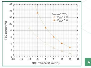
Power consumption of the built-in TEC<sup>1</sup> as a function of the QCL chip temperature for a base plate temperature of +40°C, with and without a thermal load in the QCL.
