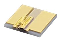
SemiNex delivers the highest available power at infrared wavelengths between 12xx and 19xx nm. When necessary we will further optimize the design of our InP laser chips to meet oustomers' specific optical and electrical performance needs. Diodes, bars and packages are tested to meet customer and market performance demands. Typical results and packaging options are shown. Contact SemiNex for additional details or to discuss your specific requirements.
