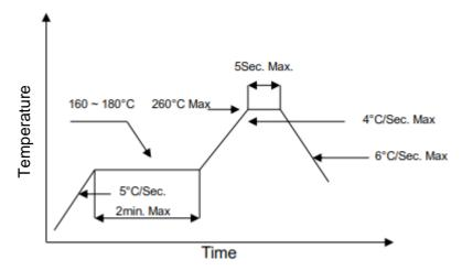
Note: Reflow soldering can be operated only one time. During the temperature ramp-up, no forces
