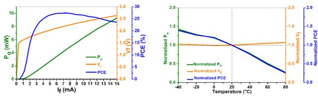
**Note:** 1. LIV graph was measured at 25 °C (left); power output, voltage and power conversion efficiency variation trend with changed operating temperature (right, normalized).
