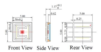
VD-0850I-006W-1F-2A0 with Substrate 1=AIN and Package F=6868 (unit: mm)
