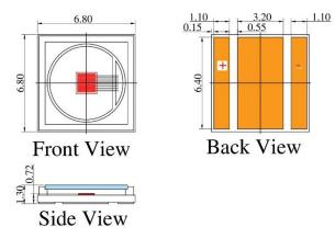
VD-0850I-006W-6K-2A0 with Substrate 6=Cu and Package K=T-mount (unit: mm)
