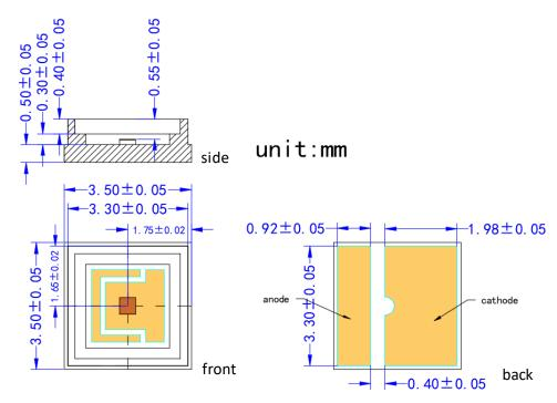
VD-0850I-002W-3E-2A0 with Substrate 3=<u>Cu/Aq</u> and Package E=<u>7060</u> (unit: mm)
