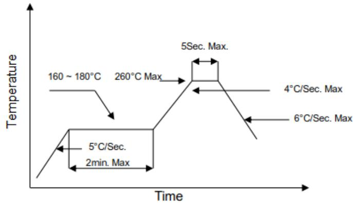
**Note:** Reflow soldering can be operated only one time. During the temperature ramp-up, no forces may be exerted on the diode which could deform or damage them. After soldering completed, please also do not process until the product temperature ramp down to room temperature.
