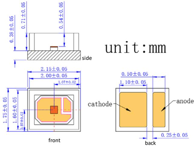
VD-0940V-140M-1C-2B0 with Substrate 1=AlN and Package C=3535 (unit: mm)
