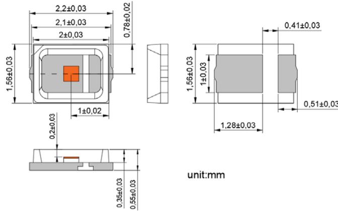
VD-0940V-140M-1A-2B0 with Substrate 1=AlN and Package A=2016 (unit: mm)
