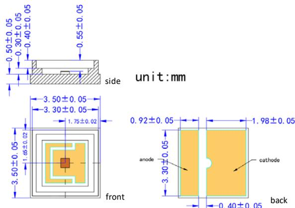
VD-0940V-140M-3C-2B0 with Substrate 3=Cu/Ag and Package C=3535 (unit: mm)
