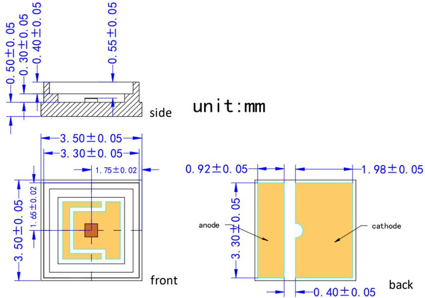
VD-0940C-070M-3C-2A0 with Substrate 3=Cu/Ag and Package C=3535 (unit: mm)
