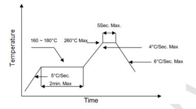
**Note:** Reflow soldering can be operated only one time. During the temperature ramp-up, no forces may be exerted on the diode which could deform or damage them. After soldering completed, please also do not process until the product temperature ramp down to room temperature.
