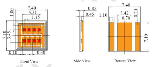
VD-0808I-020W-6K-2A0 with Substrate 4=P/Cu and Package K=T-mount (unit: mm)
