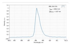
Typical spectrum of 0808 nm diode laser. Measured with 20 pm resolution.
