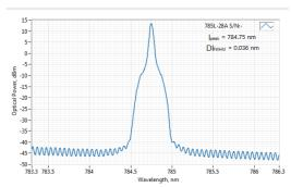
Typical spectrum of 0785 nm diode laser. Measured with 20 pm resolution.
