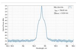
Typical spectrum of 0785 nm diode laser. Measured with 20 pm resolution.
