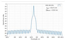
Typical spectrum of 0633 nm diode laser. Measured with 20 pm resolution.
