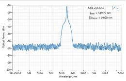
Typical spectrum of 0520 nm diode laser. Measured with 20 pm resolution.
