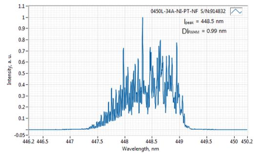
Typical spectrum of 0450 nm diode laser. Measured with 10 pm resolution.
