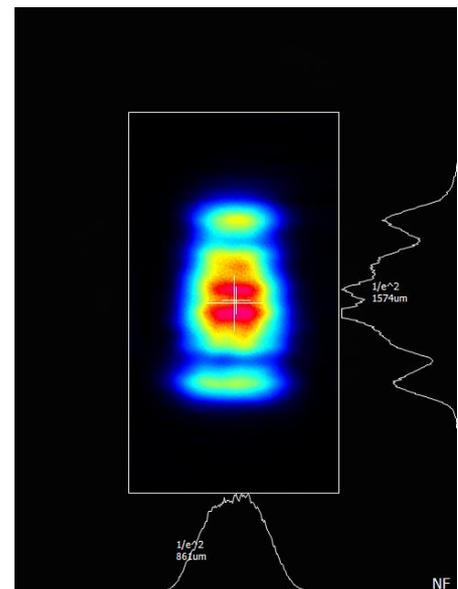
Typical near field (0.45 m from output aperture) beam profile. Non-circularized beam of a 0450 nm direct diode laser.
