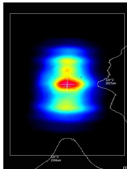
Typical far field (1 m from output aperture) beam profile. Non-circularized beam of a 0450 nm direct diode laser.
