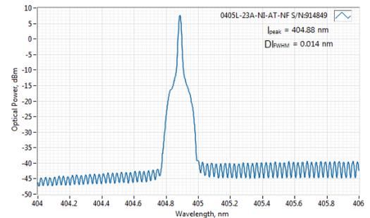
Typical spectrum of 0405 nm diode laser. Measured with 10 pm resolution.
