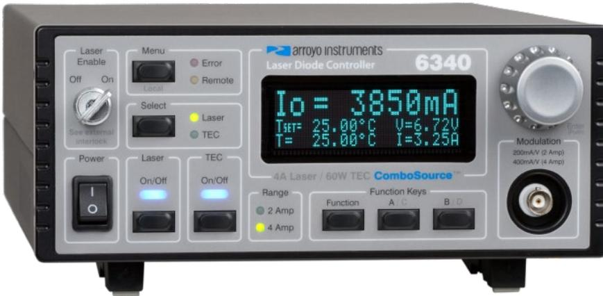
The 6300 Series ComboSource is a high-accuracy laser driver combined with a 60W temperature controller. With unique operational modes and safety features not found in other devices, this instrument is ideal for low and medium-power laser and LED applications.
