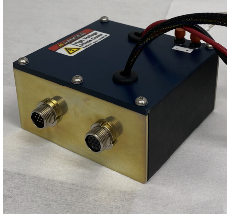
532 Laser Electronics: 3.0" x3.0" x1.5"
