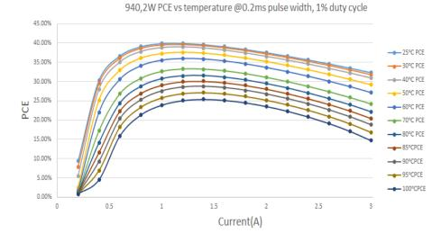
Optical power vs temperture @0.2ms pulse width, 1% duty cycle
