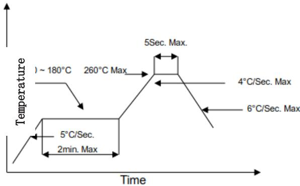
Note: Reflow soldering can be operated only one time. During the temperature ramp-up, no forces may be exerted on the VD which could deform or damage them. After soldering completed, please also do not process until the product temperature ramp down to room temperature.
