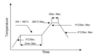
Note: Reflow soldering can be operated only one time. During the temperature ramp-up, no forces may be exerted on the LD which could deform or damage them. After soldering completed, please also do not process until the product temperature ramp down to room temperature.
