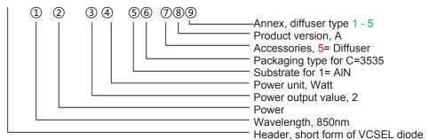
Part (9) (Diffuser beam angle) Option to choose specific diffuser types
